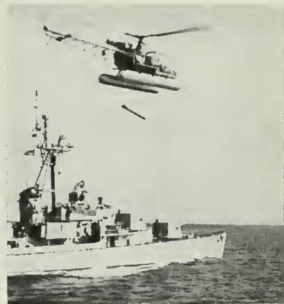
DUMMY homing torpedo is dropped by jet copter based on destroyer.
